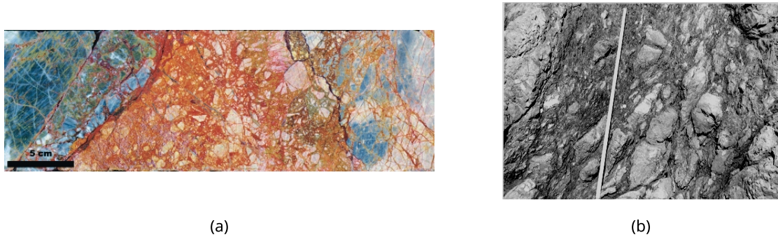
Figure 3.1: Images of exemplary bimrocks: (a) Transition from blocky rock mass into bimrock (central part of picture); mesoscale (from [324, Fig. 7, p. 18]). (b) Franciscan mélange showing anisotropic fabric of elongated blocks entrained within sheared shale matrix; scale bar is 1.5 m (from [255] graphed in [253, Fig. 1, p. 600]).
